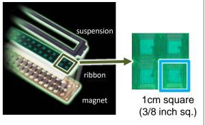
MCMA stands for Multi Cell Microtransducer Array based on planar ribbon technology. MCMA consists of multiplanar magnets and micro-cells imprinted on a diaphragm. usfps.com/index.html#mcma
